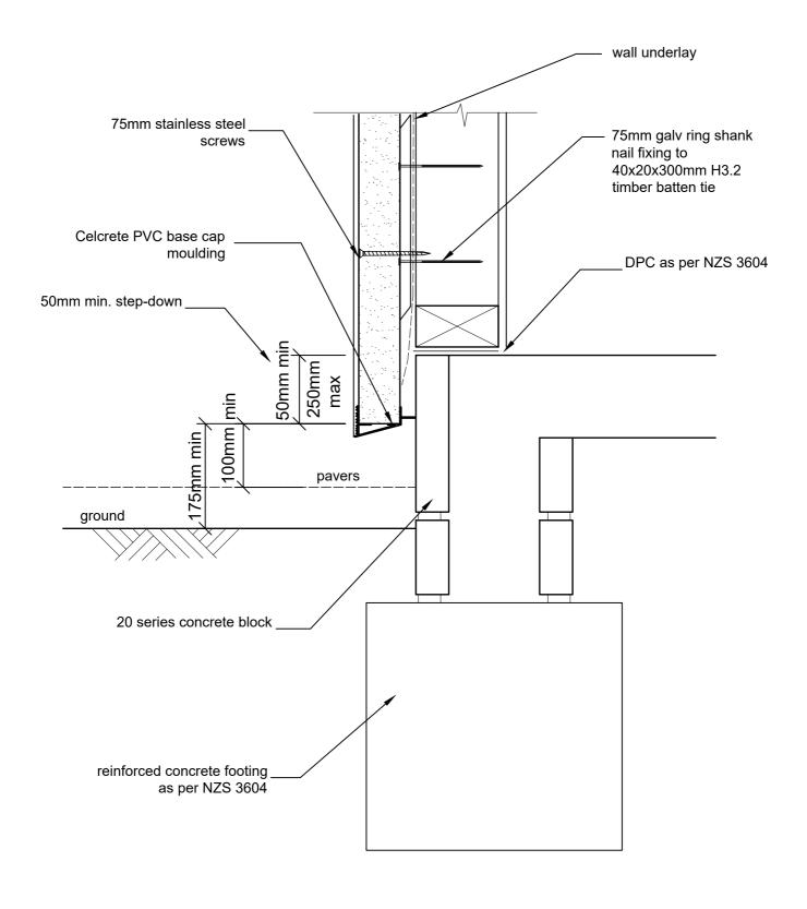
OVERHANGING FOOTING DETAIL - 20mm CAVITY CAD REF 4-2 -20 SCALE 1:5
