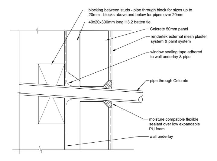
Where cables penetrate cladding, a sleeve or conduit shall be provided and sealed into the celcrete 50mm panel system. All wires that pass through a conduit shall be sealed into position inside the conduit.
