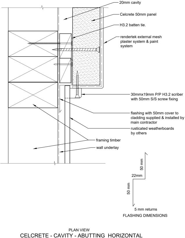
CELCRETE - CAVITY - ABUTTING HORIZONTAL TIMBER WEATHERBOARDS
