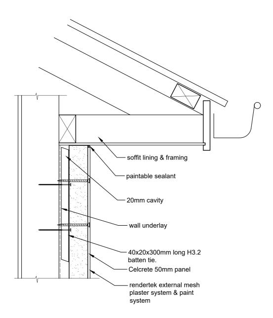
CELCRETE PANEL SOFFIT EAVES JUNCTION DETAIL - 20mm CAVITY CAD REF 8-6-20 SCALE 1:5
