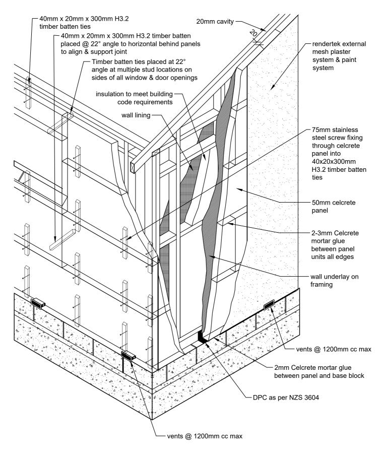
CELCRETE 50mm PANEL VENEER SYSTEM FIXING DETAILS - 20mm CAVITY CAD REF 3-1-20 SCALE 1:20 Celcrete Panel Veneer System
