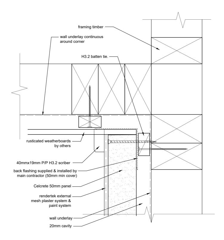
PLAN VIEW CELCRETE PANEL INTERNAL CORNER JUNCTION WITH HORIZONTAL TIMBER WEATHERBOARDS CAD REF 14-3-20 SCALE 1:2 Celcrete Pa
