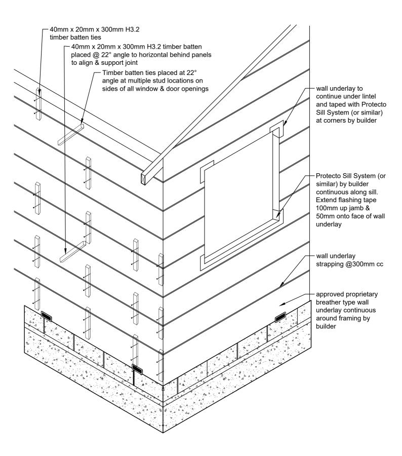
CELCRETE 50mm PANEL VENEER SYSTEM FIXING DETAILS - 20mm CAVITY CAD REF 3-1a-20 SCALE 1:20
